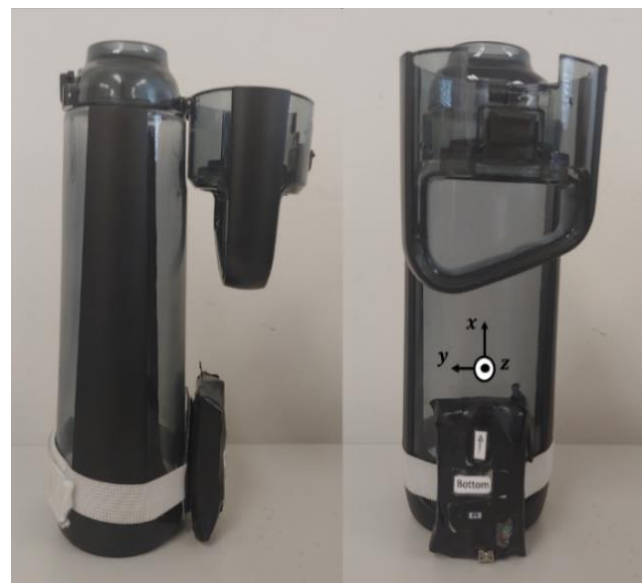
Fig. 1. Side and Back View of Sensor Attached to Bottle.
