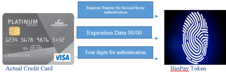
Fig. 1: Overview of the BioPay scheme architecture, which is considered to replace the current standard, which is a credit card. Each BioPay token has similar information as actual credit card such as expiration data, four digits for authentication, and a second factor authentication as a customer phone number where the BioPay scheme sends authentication messages
