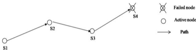
Fig. 5. Sensor Nodes Cascaded Movement after Failure.
