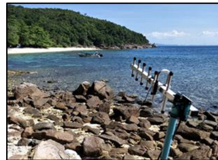
Fig. 6. The Sensor Node Connected with Yagi-Uda Antenna.
