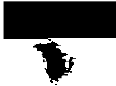
Fig. 11. Edge Segmentation: 42J Impact, 0.41 Threshold.
