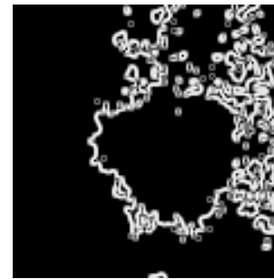
Fig. 8. Gradient Magnitude: 28J Impact, 0.67 Threshold.
