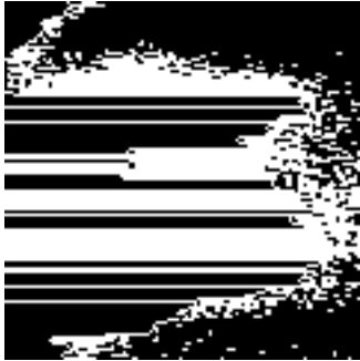
Fig. 21. Edge Segmentation 56J Impact, 0.31 Threshold (No Segmentation Possible).
