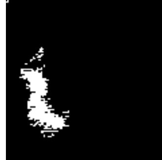
Fig. 25. Edge Segmentation 42J Impact, 0.51 Threshold (No Segmentation Possible).
