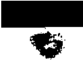
Fig. 2. Gradient Magnitude: 28J Impact, 0.57 Threshold.
