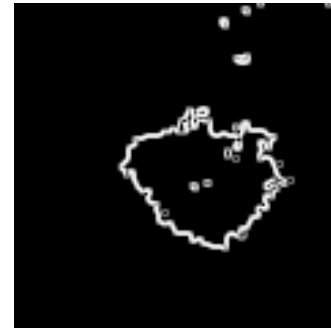
Fig. 6. Gradient Magnitude: 28J Impact, 0.61 Threshold.
