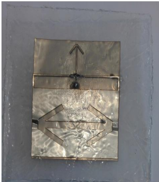
Fig. 7. Antenna manufactured using Laser Method.
