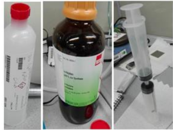
(a) silicone (b) n Heptan (c) two syringes for the liquid exchange
