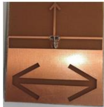
Fig. 6. Fabricated Antenna with PCB Method.
