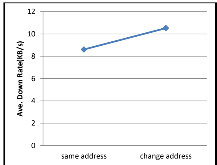
Fig. 8. Average Download Rate by One Peer for the Case of Change of Address and Without Change of Address.
