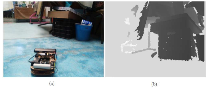
Fig. 20. Illuminated image of 10lux, (a) Real capture image, and (b) Map of disparity obtained from Fig. 20 (a).
