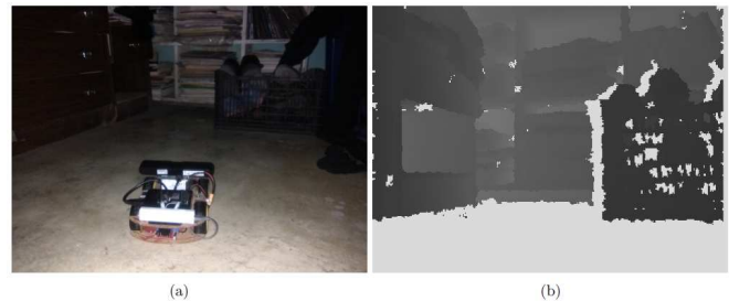
Fig. 21. Illuminated image of 0lux, (a) Real capture image, and (b) Map of disparity obtained from Fig. 21(a).
