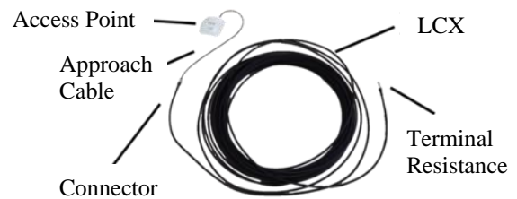
Fig. 3. An LCX Network Equipped with TCP/IP-Compliant Access Points.
