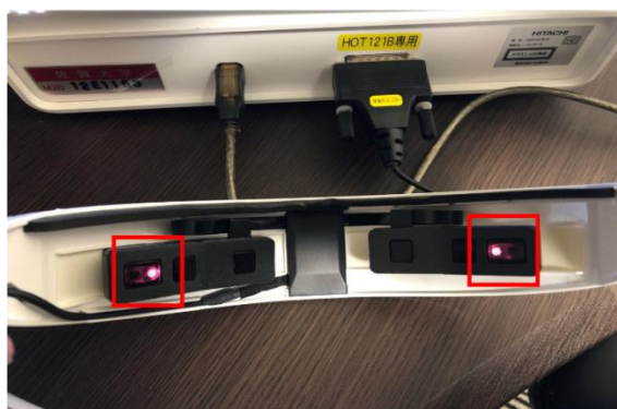
Fig. 5. Close-up Photo of the NIRS Sensors of the HOT 121B.
