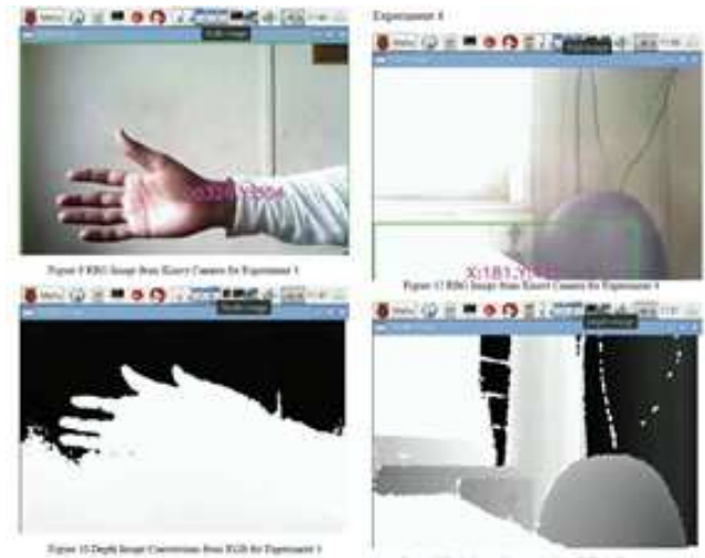
Fig. 6. Object detection using stereo vision together with Kinect [4].
