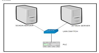
Fig. 3. Network Connectivity Diagram of Test Set up.
