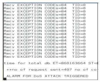
Fig. 8. DoS Attack was Detected in SCADA.
