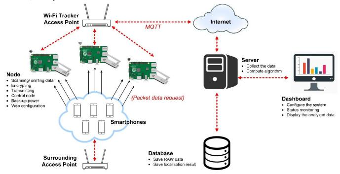
Fig. 1. Wi-Fi Tracker System Architecture.
