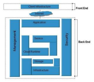
Fig. 1. Cloud Computing Architecture [31].
