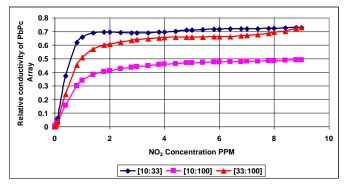
Fig. 6. Predicted and optimized sensor response for array 1
