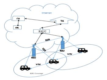
Fig. 1. IOV System Architecture.
