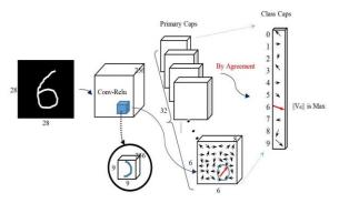
Fig. 1. CapsNet Architecture.
