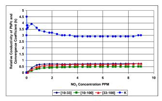
Fig. 8. Predicted Sensor Response and Convergence Coefficient for Array 1.
