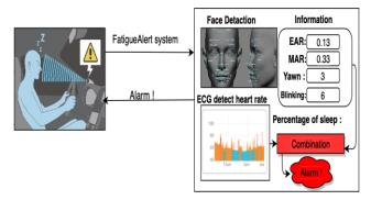
Fig. 6. A Visual Example of Built HybridFatigue Detection System using Multi-Cams Approach and Hybrid Visual and Non-Visual Features.
