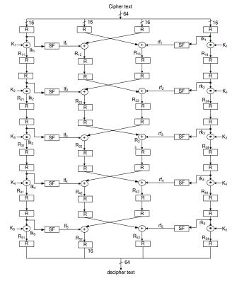
Fig. 4. Architecture of Decryption Module.
