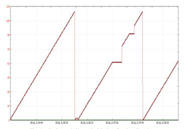
Fig. 4. DoS Attack Shown in SCADA Graph or Trend.
