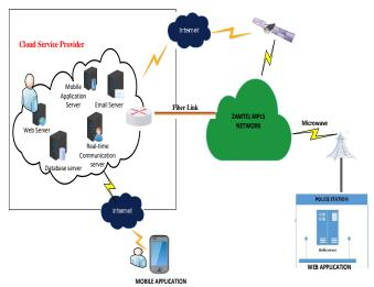
Fig. 6. Proposed System Architecture.
