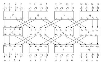
Fig. 2. Architecture of S-BOX Function (SF).
