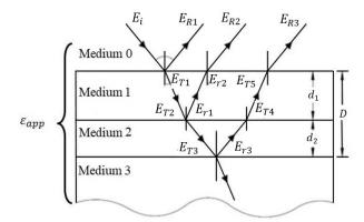
Fig. 1. Multilayered Soil Reflection Model [8].
