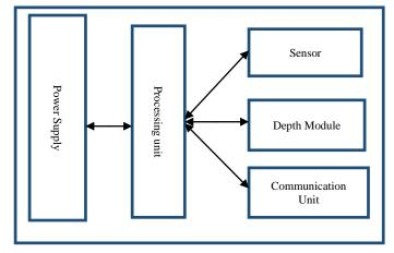
Fig. 1. Internal Architecture of underwater Node.
