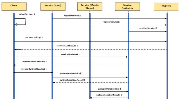
Fig. 4. The Service Distribution Sequence Diagram.
