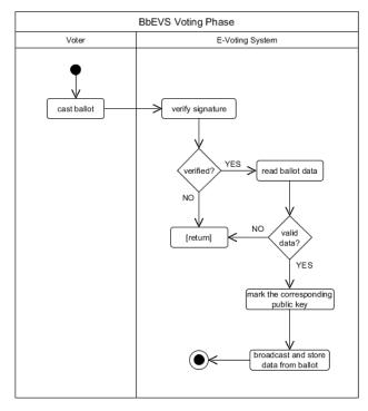
Fig. 4. Diagram of vote casting phase
