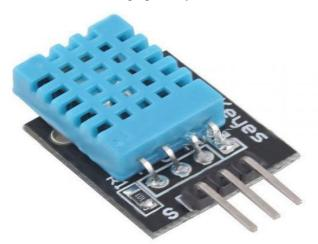
Fig. 3. DHT11 for Humidity and Temperature.
