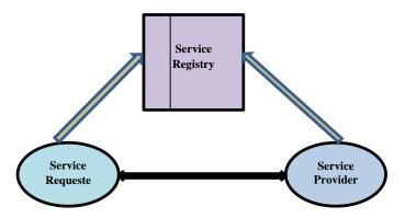
Fig. 2. The Service-Oriented Architecture.
