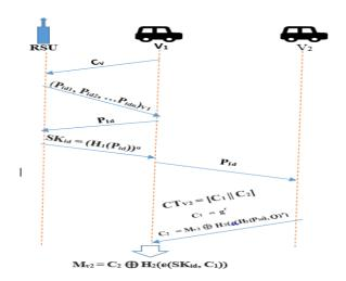
Fig. 3. Message Encryption and Decryption.
