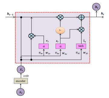
Fig. 3. Architecture of Variant E-GRU.
