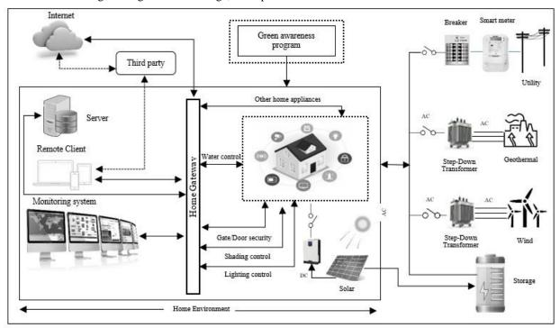
Fig. 2. Integrated Home Automation Conceptual Architecture.
