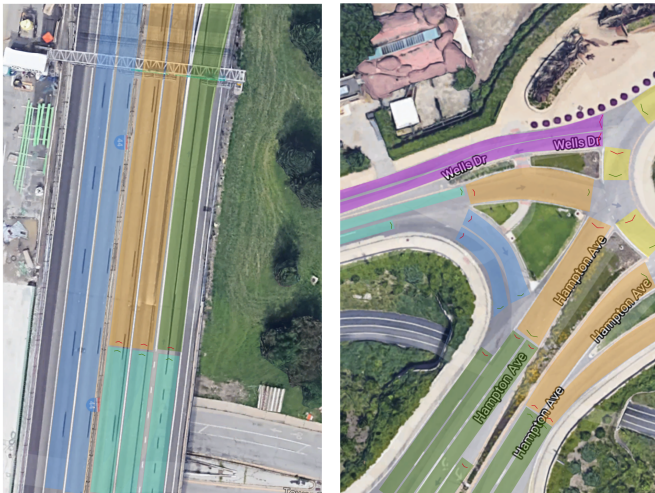
Fig. 3. An Illustration of Lane Sets under Two different Situations Overlapping on a Satellite Map, the Left is on Highway Exit, the Right is a Complicated Lane Topology near a Roundabout, the Red and Green arrows Represent Entrances and Exits of those Lanes.
