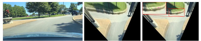
Fig. 12. Detecting the Inner Side of the Roundabout is an Example of Detecting a Special Line with only its Direction Given. The Top 2 Results are shown as Red and Blue in the Last Image in the Red Box.
