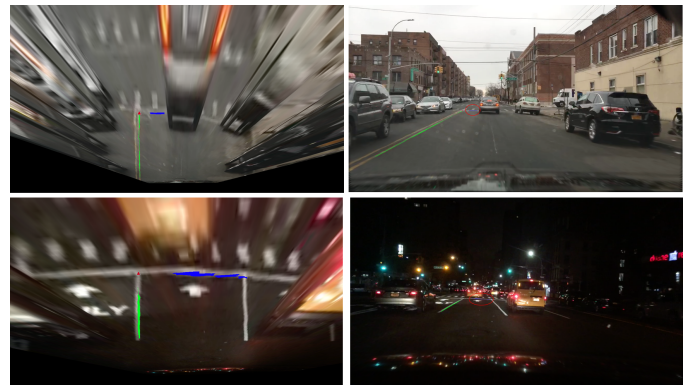
Fig. 11. Stop Lines Detected Results on BDD 100K Dataset. Blue Pixels are the Detected Stop Line and Green Pixels are the Guiding Lane Line of that Stop Line.
