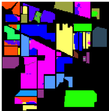
Fig. 8. Classified Hyperspectral Image using SVM and Guided Image Filter.
