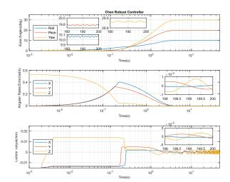
Fig. 7. Euler Angles and Angular Rate Errors produced by the miscellaneous disturbance torque in the Controller defined in (52) with a settling time (ts) of 2.75,  $\pm$  0.01 degrees in the Euler Angles oscillations, 0.2 Euler Angles offset,  $\pm$  0.7  $\times 10^{-3}$  rad/s oscillations in angular rates, and  $\pm 2.1 \times 10^{-3}$  Nm in Control Torque.
