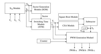
Fig. 3. Proposed Hardware Architecture of DSV-PWM Module.
