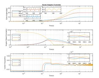
Fig. 6. Euler Angles and Angular Rate Errors produced by the miscellaneous disturbance torque in the Controller defined in (41) and (45) with a settling time (ts) of 6.48,  $\pm$  0.05 degrees in the Euler Angles oscillations,  $\pm$  2.0  $\times 10^{-3}$  rad/s oscillations in angular rates, and  $\pm 2.1 \times 10^{-3}$  Nm in Control Torque.
