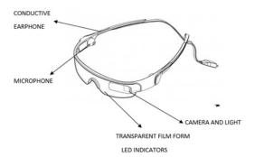
Fig. 3. Design of the Electronic Glasses
