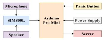
Fig. 2. The Block Diagram of our Device. The Block Diagram shows all the Hardware we have used to Develop our Safety Device.
