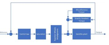
Fig. 3. Block diagram for a CubeSat subject to gravity gradient torque, and misalignment. The control law block may have adaptation algorithms depending on the simulated control law.
