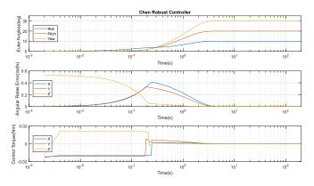
Fig. 12. Euler Angles, Angular Rate Errors, and Control Torque produced by the Chen Robust Controller defined in (52) with a settling time (ts) of 2.75 s and an average computational cost (O) of 0.309 ms. The Control Torque saturation time was 235 ms.
