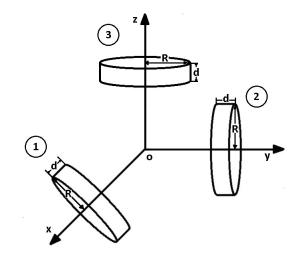
Fig. 1. Distribution of the reaction wheels described in the body frame which origin coincides with the center of mass and geometric. The loads are considered to be fully balanced around the 'o' origin. Adapted from [2].
