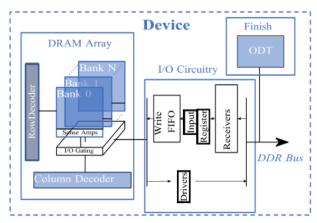
Fig. 3. General Overview of DRAM Device Structure.
