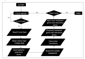
Fig. 1. Flowchart of DTO Optimisation Process.
