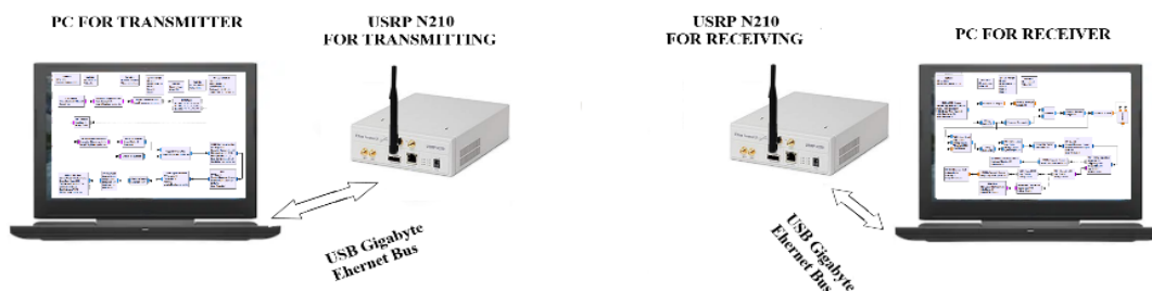
Fig. 5. Image of the Test Set-up for a Real-Time Radio System.
