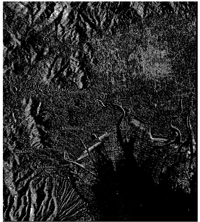
Fig. 13. Subtracted Image between Ortho Rectified VV Sigma Note (Back Scattered Cross Section of the Earth Surface) in unit of Decibel of the Areas which are Acquired on 20 September and 1 October.
