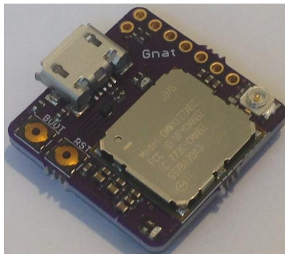
Fig. 3. CMWX1ZZABZ LoRa Module used for Data Transmission between Smart Meter units and Local Monitoring Centre.
