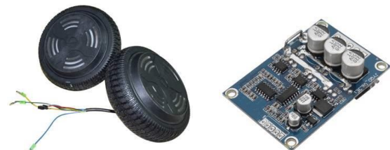
Fig. 5. Three-Phase Brushless DC Motor with Motor Diver.
