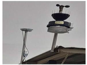
Fig 2. The Weather Station VISIOGREEN with Pyranometer.
