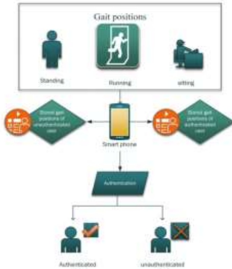
Fig. 4. GAIT Verification Process.
