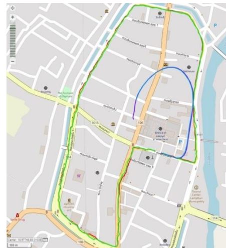
Fig. 7. GPS Positions after all Three Sensors were Measured for Averages and Implemented with Kalman Filter Every N Term, and after Data from all Three Sensors were Implemented with Kalman Filter and then Measured for Averages in the Case that the Equipment was Continually Moving.
