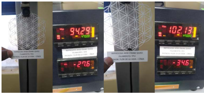
Fig. 14. Tensile and Elongation Tests of Flower of Life Pattern with Line, Printed with TPU and TPE Flexible Filaments.
