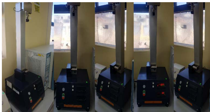
Fig. 3. Dynamometer Model 848 from J. Bot S.A. used in Tensile and Elongation Tests of the Printed Natural Patterns.
