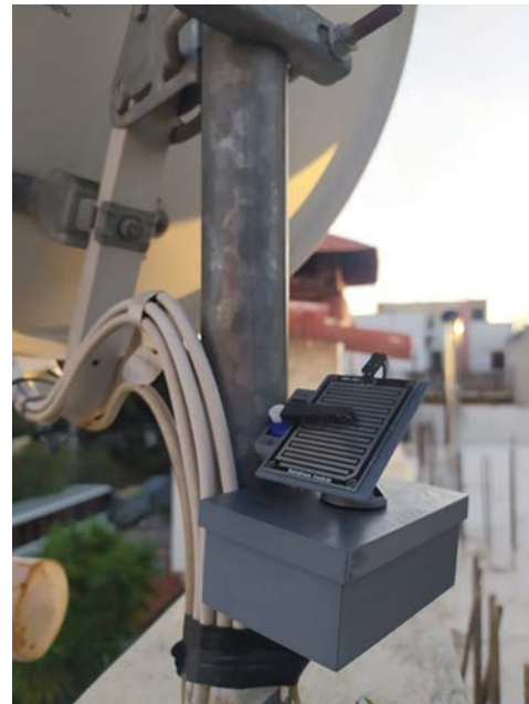
Fig. 6. IoT based Rainfall Monitoring System with 3D Case.
