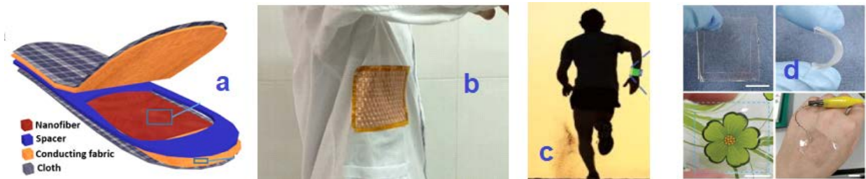
Fig. 5. Applications of TEEH: (a) Smart Shoes [33], (b) Smart Cloths [42], (c) Smart Watch [43], (d) Smart Skin [45].
