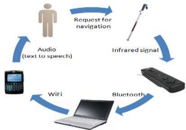
Fig. 5. Components of the Navigation System [7].
