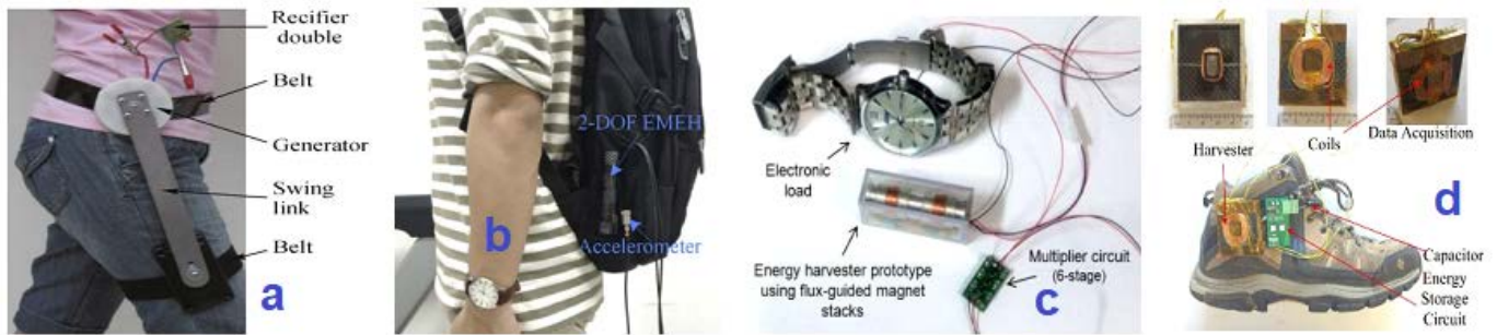
Fig. 7. Applications of EMEH: (a) Hip Mounted Leg [48], (b) Smart Arms [60], (c) Smart Wrist Watch [68], (d) Smart Shoes [69].
