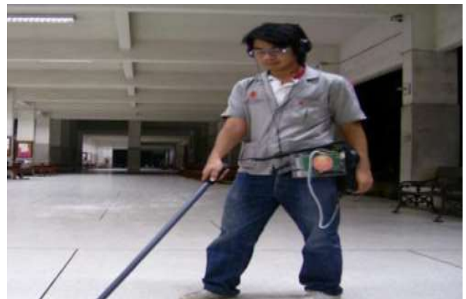
Fig. 6. Navigation Device Attached to a user with a Headphone and a Cane with a Built-in RFID Antenna [8].
