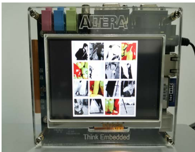
Fig. 10. Real Live Implementation of Second Splitting on NEEK Board.
