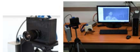
Fig. 4. MSFA One-Shot Camera.
