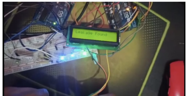
Fig. 12. Leakage Found Message Display.
