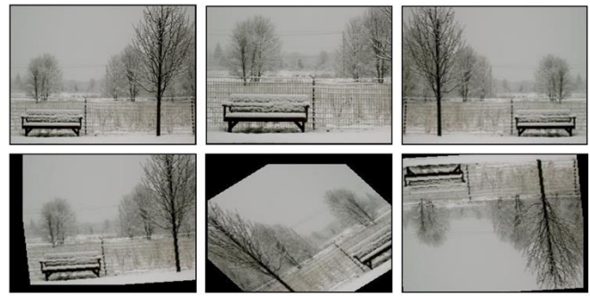
Fig. 3. Different Methods of Data Augmentation Including Rotation, Flipping, Translation, and Cropping and Resizing.
