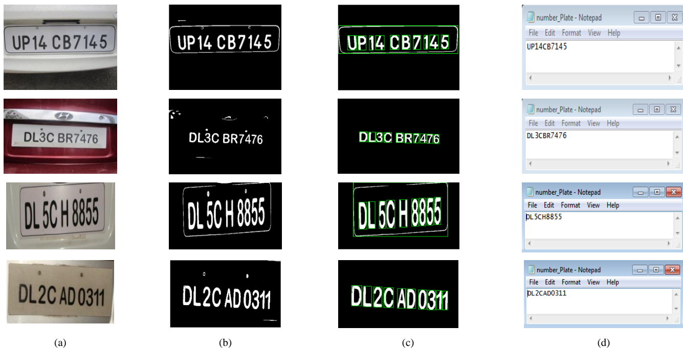
Fig. 5. (a) Original Image (b) Binary Image (c) Boundary Box for Character Segmentation (d) Recognized Number Plate Value.
