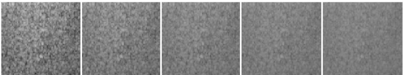
Fig. 2. Diagram Showing the Results of Adding a Constant Intensity Bias to the Original Image Shown to the Left. The Speckle Pattern Detectability Decreases As Intensity Bias Increases From Left to Right Images.
