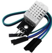
Fig. 6. DHT22: Temperature and humidity module
