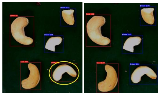
(a) Detection result of YOLOv7E6E (b) Detection result of YOLOv7tiny Fig. 5. Comparing YOLOv7tiny and YOLOv7E6E cashew detection results in weak light conditions
