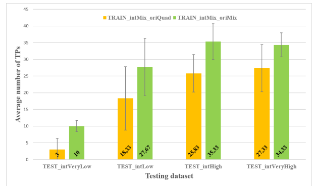
Fig. 12. Comparisons of the average numbers of TPs on the test subsets arranged by brightness, grouped by light orientations within their training data
