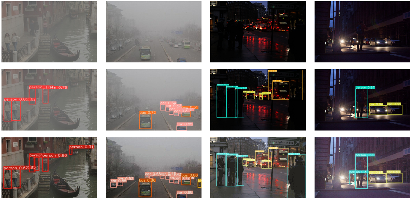
Fig. 4. Visualization. Detection results of YOLOv5 (middle row) and PDE (bottom row) on RTTS (columns 1, 2) and ExDark (columns 3, 4). PDE achieves better object detection accuracy and better visualization for the user in low visibility images.
