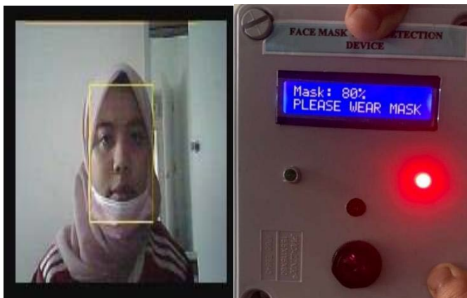
Fig. 8. The Device Displays "Please Wear the Mask".
