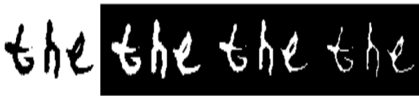
Fig. 2. The Thresholding of Word Image after Applying the Negative and Line-thinning Operations.
