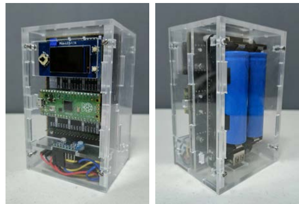
Fig. 1. Goniopi with Assembled Digital Goniometer in the Acrylic Case.
