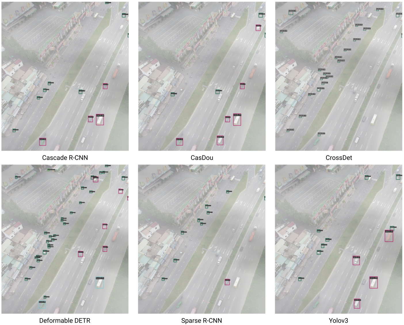
Fig. 9. Visualization Images of Detectors on UIT-DroneFog Dataset. (In Order to See the Image Clearly, Please Zoom in 2×.)
