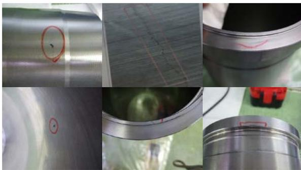
Fig. 1. Common Surface Defects of Cylinder Liner. From the Upper Left to the Lower Right, they are the Sand Defect, the Crack Defect, the Wear Defect, the oil Defect, the Scratch Defect and the Collision Defect.
