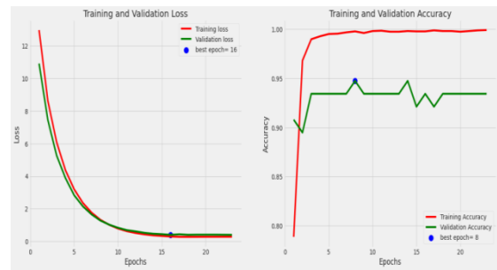
Fig. 9. Model Performance for 10 Pest Classes based on Faster R-CNN Efficient Net B4.
