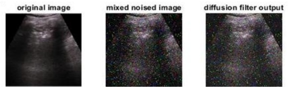
Fig. 7. Simple AD Filter (a) Original pneuLung POCUS Image (b) Image Corrupted by Mixed Gaussian Impulse Noise ( \sigma=0.02 and \rho=0.02 ) (c) Response of Simple AD Filter.
