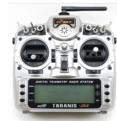
Fig. 4. Fr-sky taranis radio transmitter/radio controller
