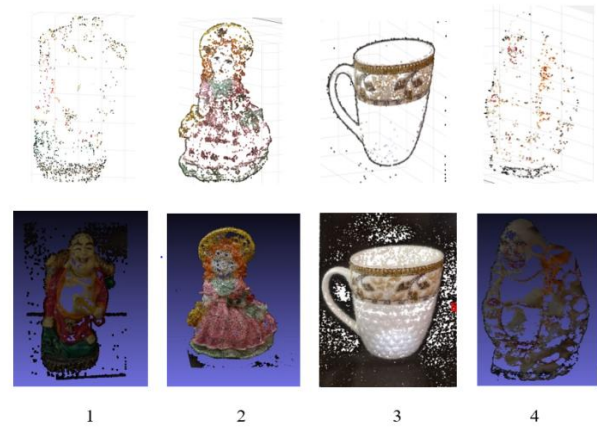
Fig. 3. 3D point cloud of object Image (row1 sparse point cloud, row 2 dense point cloud).
