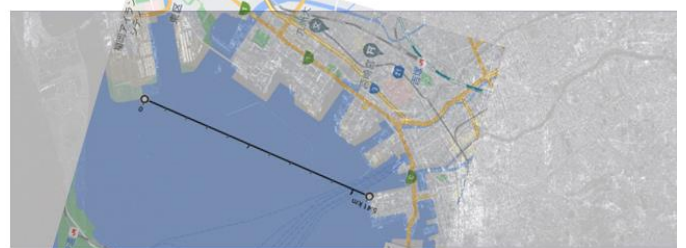
Fig. 3. Locations of GCPs and the distance between two GCPs (Fukuoka).
