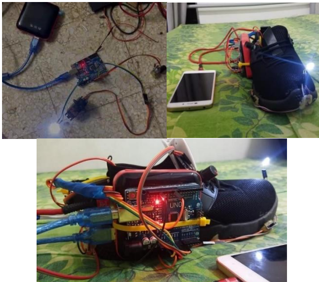
Fig. 9. Auto lacing and light circuit connection.
