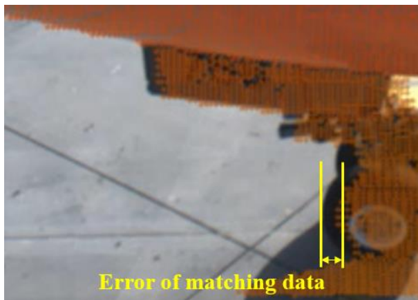
Fig. 13. Image-LiDAR matching deviation data results (Aircraft landing gear).
