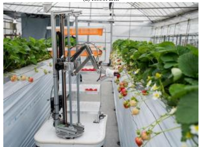
(b) Robot at work harvesting
