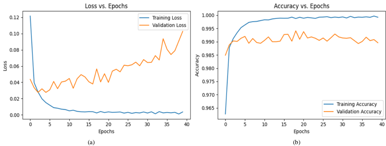
Fig. 7. Loss versus accuracy curves for training and validation with respect to epochs for pro-posed depressive-deep system, where figure (a) shows the training and validation loss curves, (b) represents the training and validation accuracy curves.
