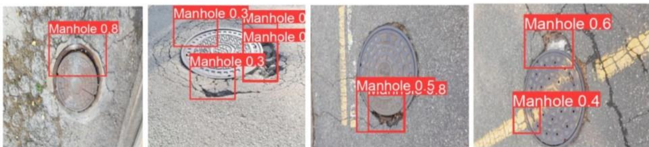
Fig. 7. Examples of wrongly detection of manholes cover using YOLOv8.
