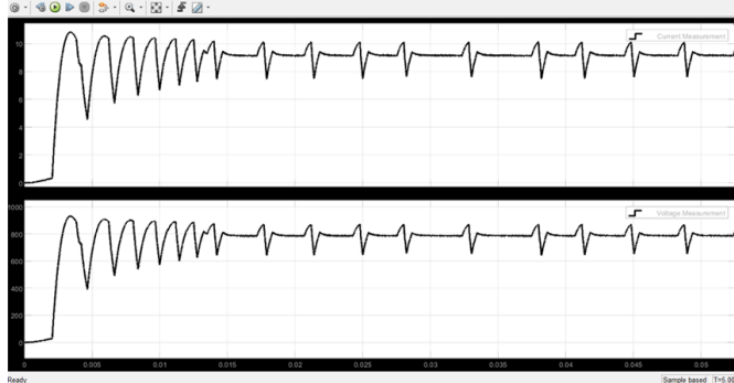
Fig. 11. Fluctuations of current and voltage values at the exit of the booster in the PD controller scheme.
