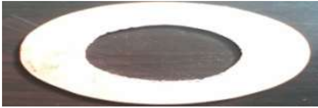
Fig 11 view of fabricated ground plane of MHD antenna with copper coating.
