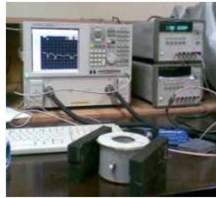
Fig 6 complete set for measurements of VSWR on MHD antenna with additional magnetic field
