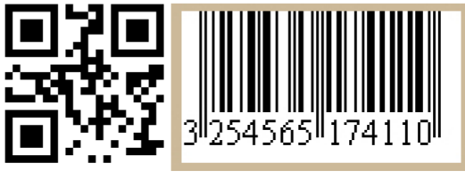
Figure 5. QR Code (2D) and EAN-13 (1D) barcodes encoding the same data (3254565174110)[6].
