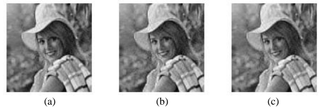
Figure 11. Reconstructed Image From 30 SVD truncated components (a) its SVs (b) SVs of figure(10a) (c) SVs of figure(10b)
