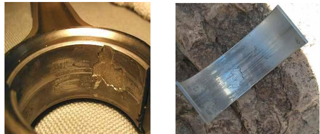
Fig. 8. Fault of bearing.
