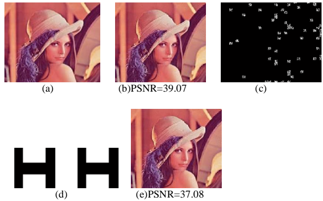
Fig. 12 a)Original image, (b) Watermarked image, modulation factor( m_k )=0.5, (c) Added watermark, (d) Extracted watermarks, (e) Watermarked image, modulation factor( m_k )= 0.7.
