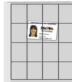
Fig.6. Outline of how a rectangular grid is applied on the entrance image to localize the watermark location.
