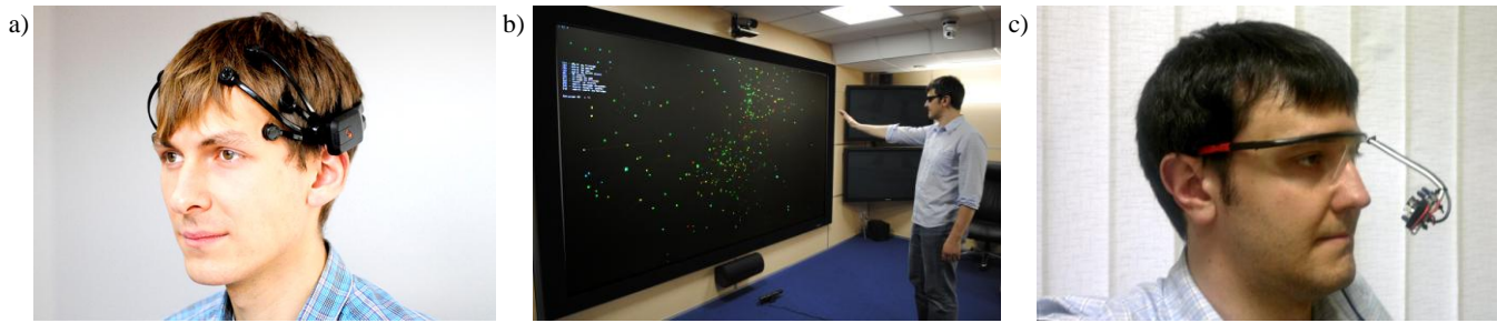
Fig.1. Experimental facilities: a) Emotiv EPOC BCI; b) 3D-Wall and Microsoft Kinect; c) DIY eye-tracking system
