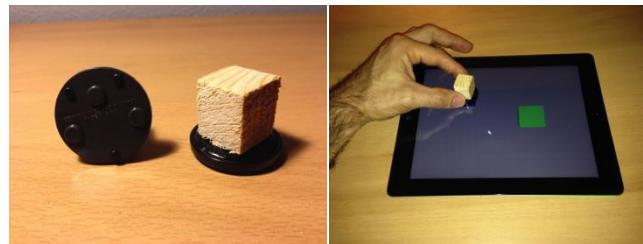
Fig. 6. A tangible cube used to create a virtual cube in the prototype.
