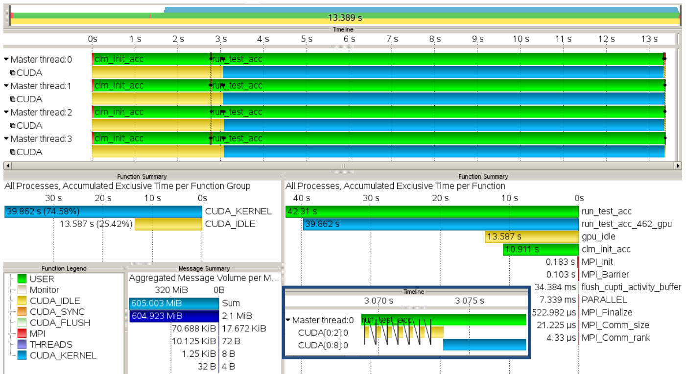
Fig. 7. Vampir visualization of CNGResp Model running on 4 Titan nodes with 4 MPI processes and 4 K20x GPUs. The main timeline is shown in the top panel. A small segment of the data movement is shown in a close-up window on the bottom. One can clearly see that the GPU is only idle when there is no data transfer or kernel execution. The Function Summary (left middle) shows that almost 75% of the GPU is fully occupied. The Function Summary (right middle) shows profile information of all functions. A Function Legend is shown on the left bottom panel. A Message Summary (left bottom) shows that 605MiB of data were copied between host and GPU device
