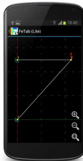
Fig. 8. Graphical Display of a 2D Truss Problem. Note display of constraint symbols on left hand side and load arrow symbols on the right.
