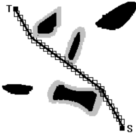
Fig. 6. The first example illustrates a path planning of a boat. Such an environment is populated by a group of islands seen as obstacles to what you can add boats supposedly immobile. The problem then is to determine the shortest path without collision from a starting point S to a point of arrival T. The obstacles are dilated by the size of the moving object (the boat in our case): the shaded area.
