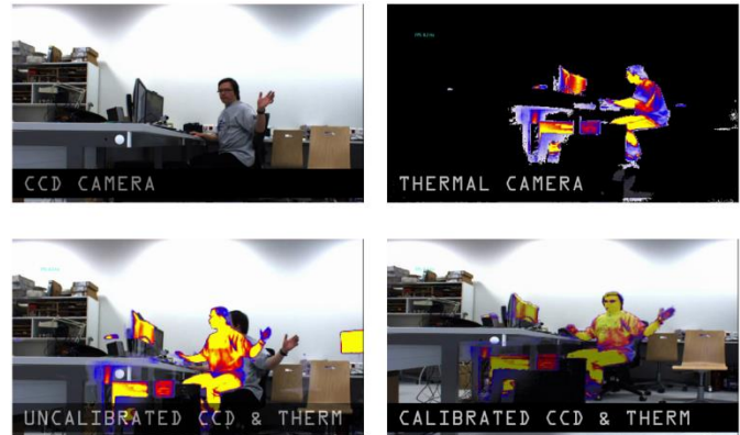
Fig. 19. Image of CCD camera (upper left), image from the thermal imager (upper right), uncalibrated data fusion (bottom left), calibrated data fusion (bottom right)
