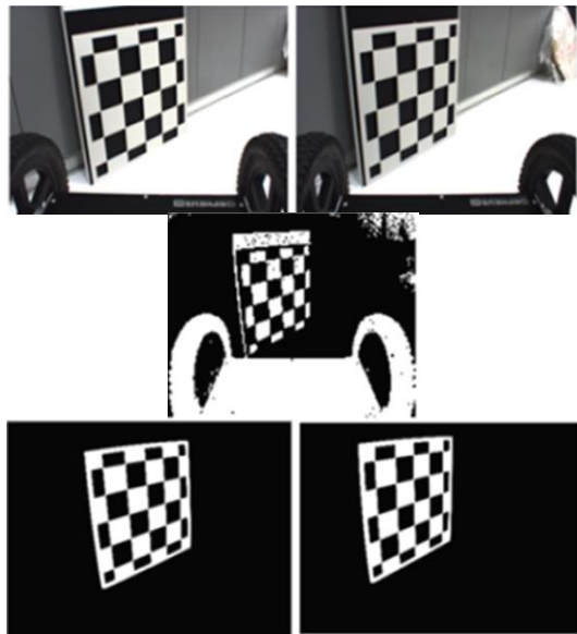
Fig. 3. The final calibration plate: the left and right CCD cameras (up); the TOF camera intensity image (center), the left and right thermal imager cameras (down)
