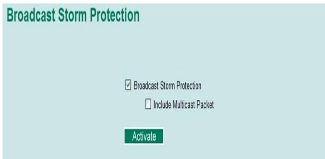
Fig. 5. Broadcast storm protection
