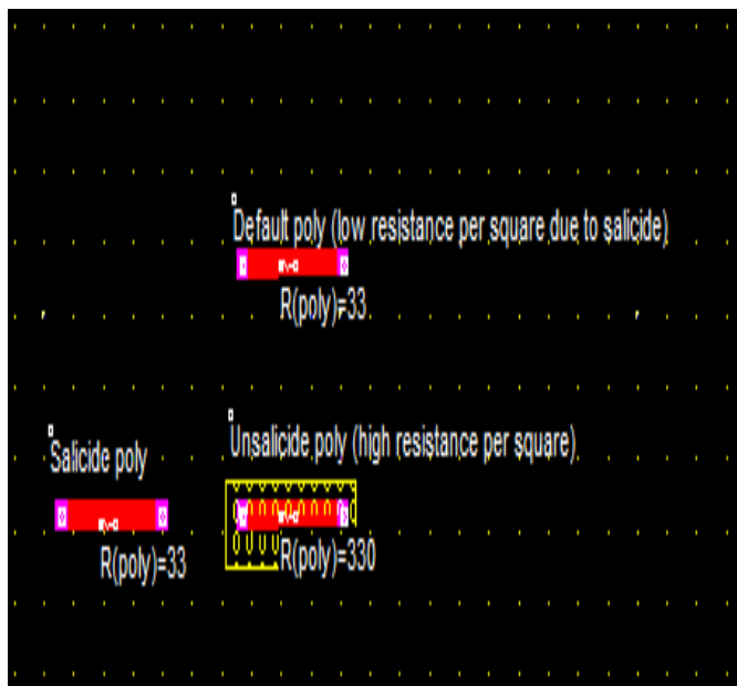
Fig. 5. Silicide material analysis in SRAM cell
