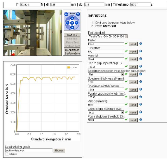
Fig. 4. Interface of tele-operated Tensile Test [6]
