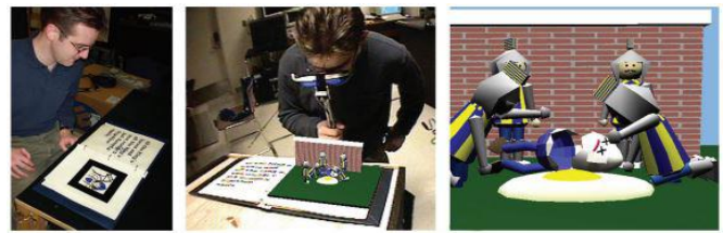
Fig. 3. Using the MagicBook interface to move between reality and virtual reality [37]
