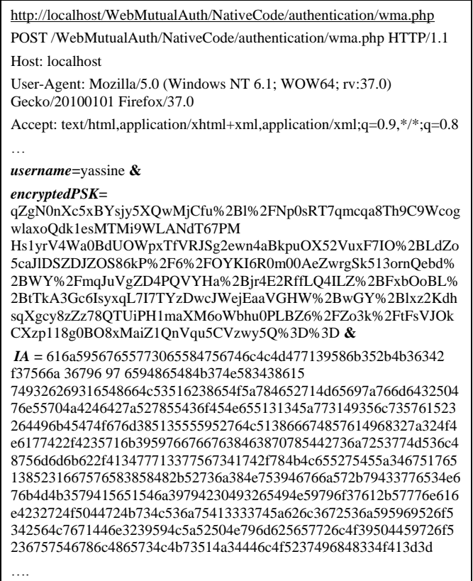
Fig. 19. Part of the HTTP request sent by the authentication extension to the web application authentication's service
