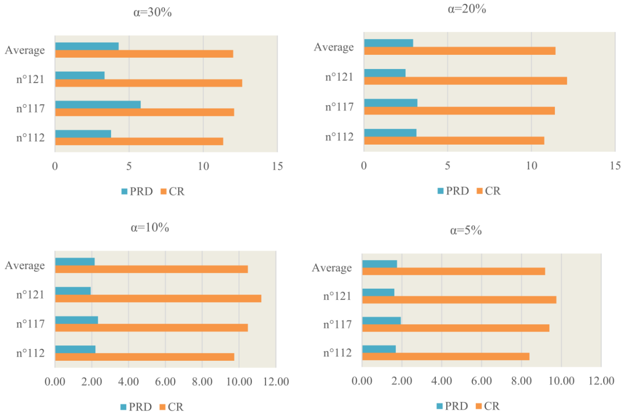
Fig. 9. CR and PRD results of the proposed method using different levels of the \alpha parameter
