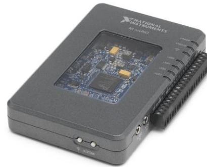
Fig. 3. Embedded NI myRIO-1900 Board
