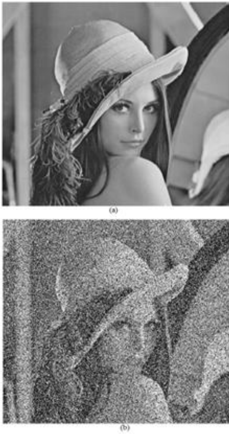
Fig. 11. Lena image: (a) original (b) with 40% salt and pepper noise.
