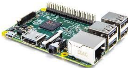
Fig. 2. Raspberry PI 2 Model B
