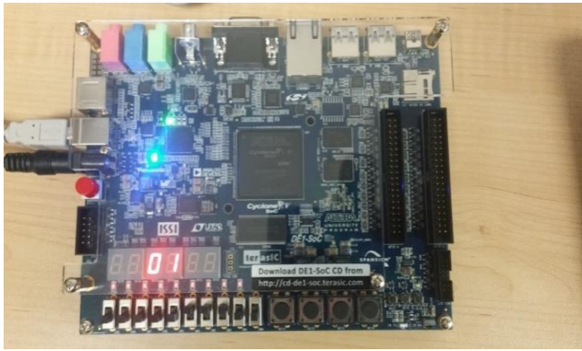
Fig. 14. The value shown on the LCD after the implementation of DE1 Altera cyclone V.
