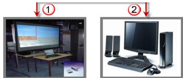
Fig. 12. Example of semi-immersion, (1) projection screen, laptop, and I-glasses; (2) conventional monitor, keyboard, and mouse, [31].
