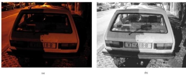
Fig. 6. The proposed shadow removal process, (a) Input image, (b) Gray scale image after shadow removal
