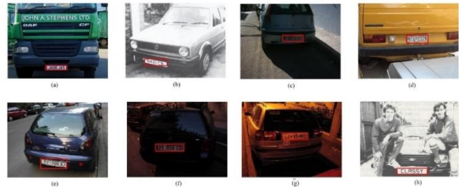
Fig. 10. Examples of license plate detection by proposed automatic license plate detection in different conditions: (a), (d), (e) day light, (b), (h) images with low contrast, (c) shaded image, (f), (g) night shot images.
