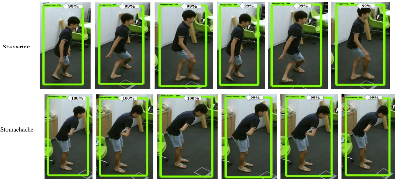
Fig. 11. Samples of The Detection Results that used TensorFlow Object Detection Notebook Technique are based on Two Pre-Trained Models (the First Three Images from the Left are based on Faster R-CNN-Resnet Model, while the Last Three Images from the Right are based on SSD-Mobilenet)) respectively. The Results Include the Bounding Detection Box for Every of the Seven Human Health-Related Actions Including (Name of the Action Class & Detection Percentage Accuracy).
