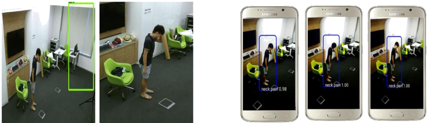
Fig. 12. Misdetectors for Some Frames of the Headache Action are based on the Pre-Trained SSD-Mobilenet (the left (Bounding Detection Box Shown in the Wrong Location), the Right (No Bounding Detection Box in the Frame)).
