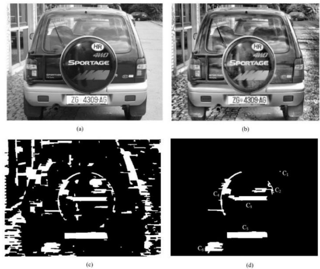
Fig. 8. The process of labeling the connected components, (a) Gray scale image, (b) Enhanced image, (c) Output image from morphological operation stage, (d) The image of the connected component based on 8 neighboring connections.
