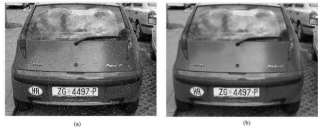
Fig. 7. (a) A noise-induced gray scale image, (b) The image after using Wiener noise filter.
