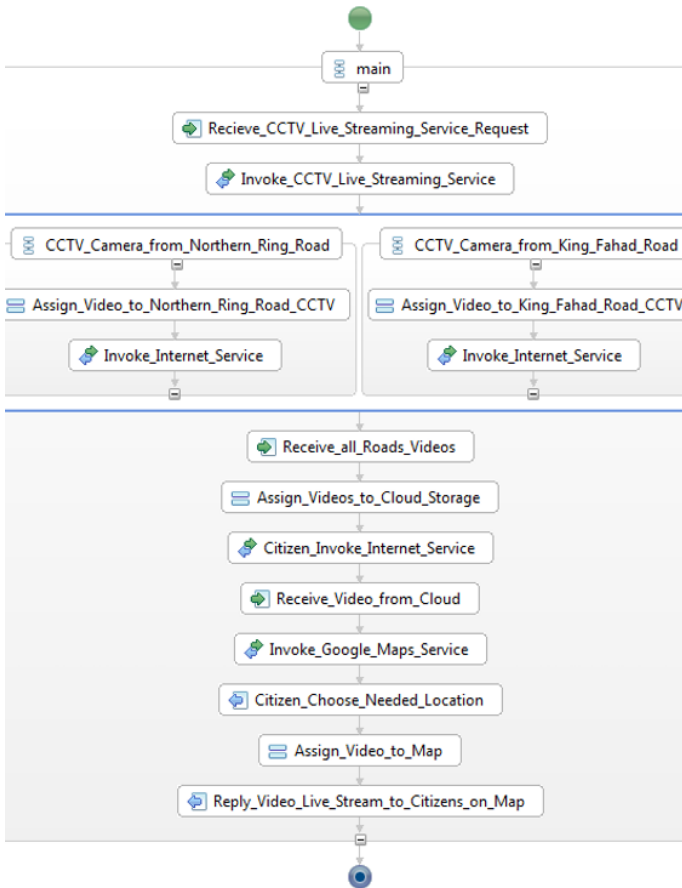
Fig. 8. CCTV Live Streaming Service BPEL Model.
