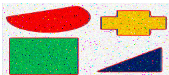
Fig. 7. Test Case 4: Noisy image having four noises, i.e. Salt & Pepper noise, Gaussian, Speckle noise and Poisson noise of variance=0.02.
