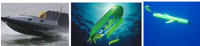
Fig. 7. a) Unmanned surface vehicle; b) Large Displacement Unmanned Undersea Vehicle, LDUUV; c) Underwater glider
