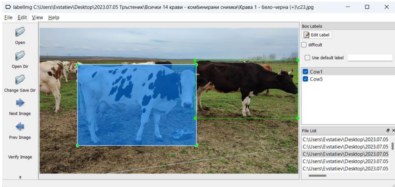
Fig. 3. Marking each object with a rectangle in the LabelImg tool.
