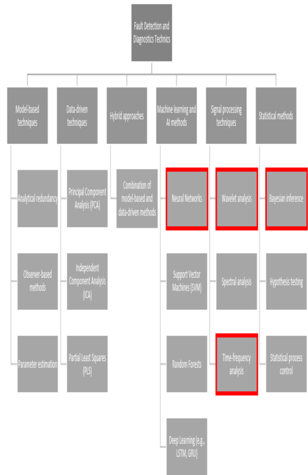
Fig. 6. Advanced techniques for fault detection and diagnostics and selected ones for the current study in red [41].
