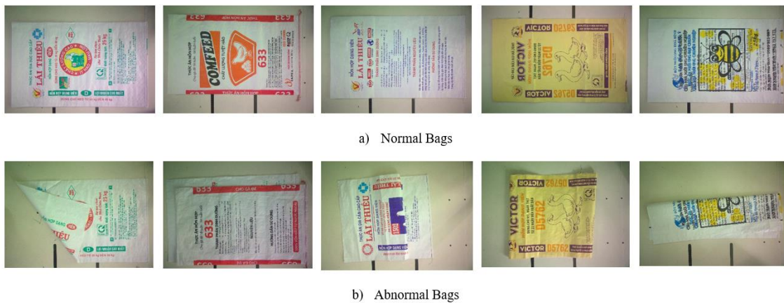
Fig. 3. Examples of normal bags (a) and abnormal bags (b).
